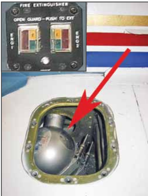
Top Left Inset: Fire Control Panel. Bottom: Engine fire extinguisher bottle in the right wing of a 421. Known instances of this system actually detecting a fire and extinguishing it are few.
