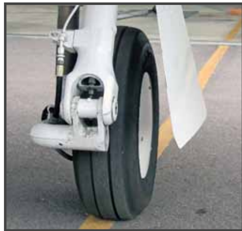
The wheel covers are slightly convex, a shape that was determined to best smooth the airflow. Plus, they look good.
