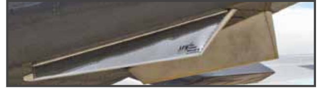
I installed strakes first and they boosted speed slightly and climb performance dramatically.
