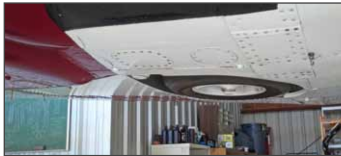
It's obvious from this picture of my airplane on jacks how the open wheel could disturb the airflow under the wing, particularly during climb.
